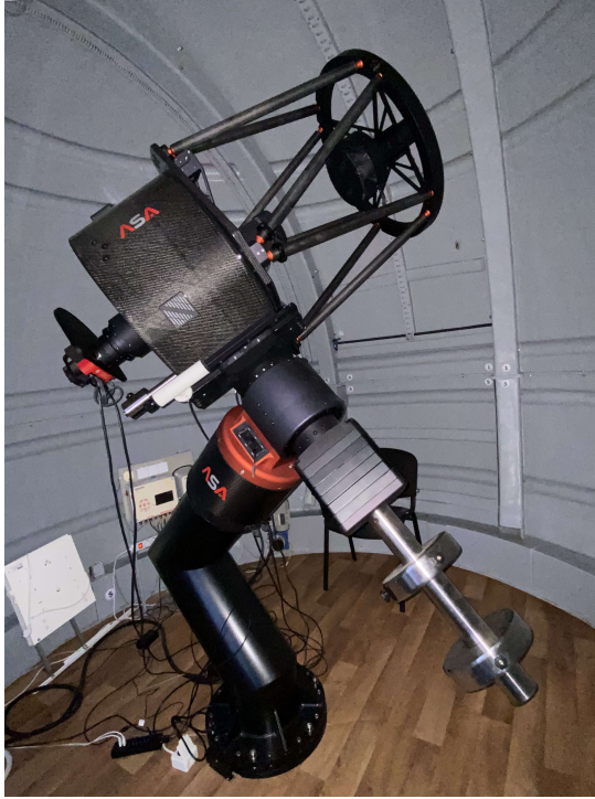
Figure 1: 60-cm Ritchey-Chretien telescope of the Shumen University
