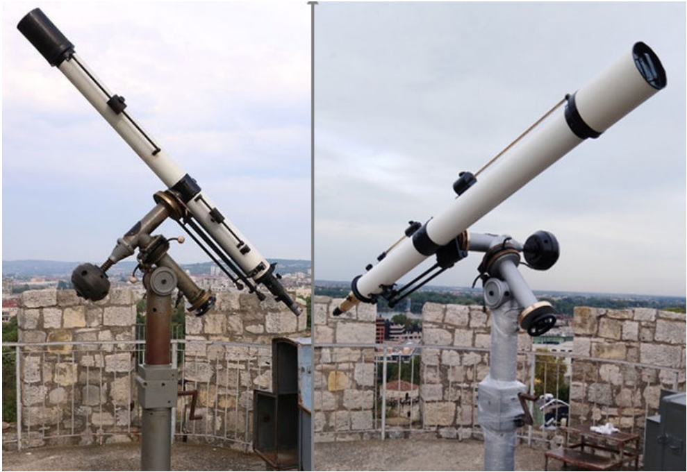
Figure 1: The Carl Zeiss Jena achromatic refractor (110/2030 mm) before (left) and after (right) the restoration.
